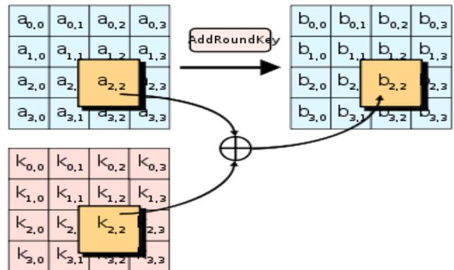
The block to be encrypted is just a sequence of 128 bits. AES works with byte quantities so we first convert the 128 bits into 16 bytes. We say "convert," but, in reality, it is almost certainly stored this way already. Operations in RSN/AES are performed on a two-dimensional byte array of four rows and four columns. Each round of the encryption process requires a series of steps to alter the state array. These steps involve four types of operations called:
